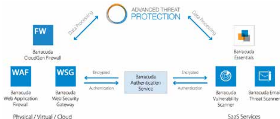
Barracuda BATP Architecture
